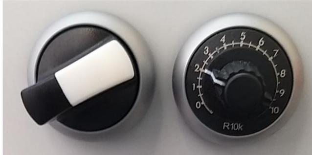
*In this example the UV-C lights will stay-on for 20 minutes (Right-hand knob on 2).*
